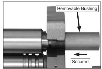
Figure 32. Securing top roller.
